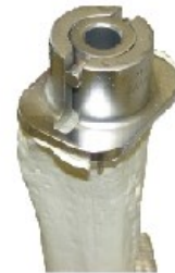
Detail of the guide for introduction of the milling cutter
