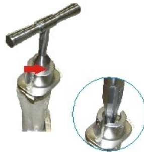
After removal of the internal guide, the manual milling cutter is deepened up to the groove shown in the detail
